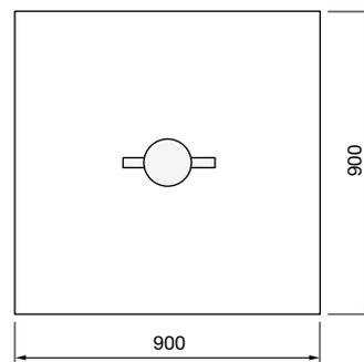
Set bollard into foundation. Fill base with concrete - capping plate has rags on underside to push into the concrete filled bollard holding plate in position once concrete has set.
