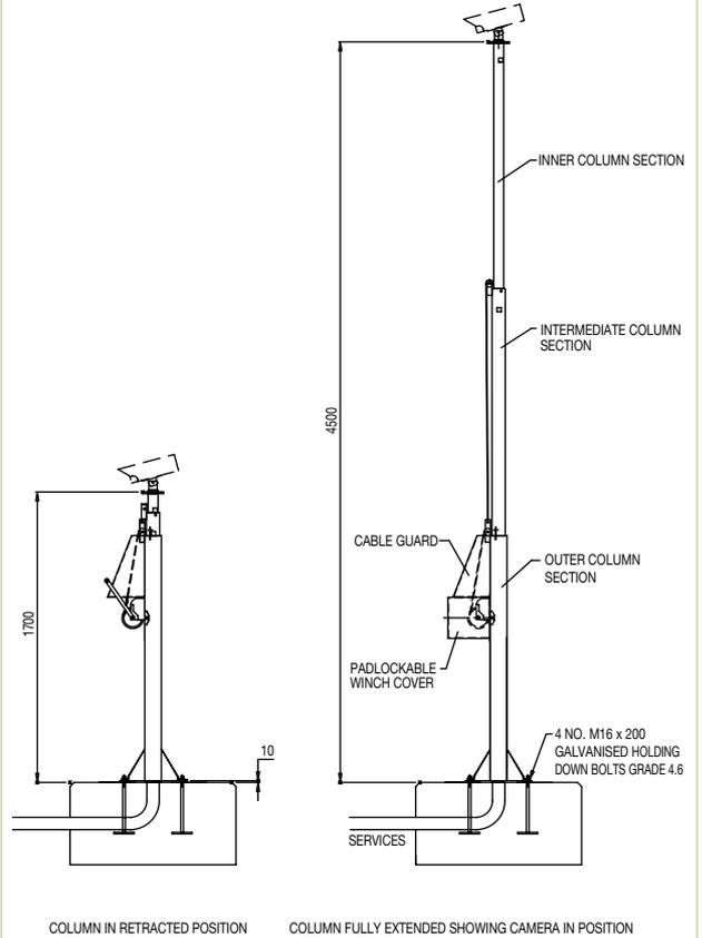
TELESCOPIC COLUMN SUITABLE FOR RESTRICTED SITE ACCESS LOCATIONS. E.G. RAILWAY YARDS/PLATFORMS WHERE CAMERA NEEDS TO BE SERVICED AT GROUND LEVEL
