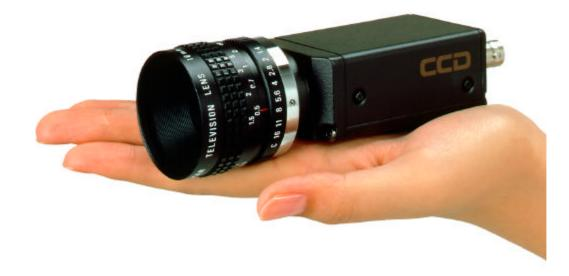
The KP-M3R is a monochrome camera using a 1/3" image size CCD with near infra red sensitivity and features high resolution and performance. Various functions are provided including multiple step electronic shutter, field on demand, integration mode switching, auto sync switching and non-interlaced scanning. The KP-M3R is suitable for a wide variety of industrial vision application including infra red microscopy and is compatible with the KP-M3
