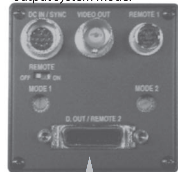
Conventional MDR-26 CameraLink Connector [39.7 x 12.9 mm]
