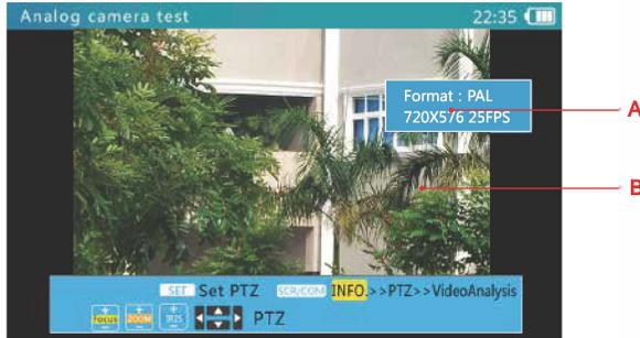
In the analog camera testing interface, it can automatically identify BNC interface signal system and resolution. Including simulation standard NTSC and PAL format signal. Simulation of the high-definition HD-CVI, HD-TVI, AHD signal format.
