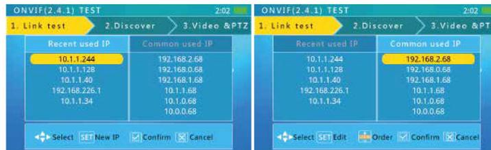
Under this mode, user can use recent IP address as static IP. On new manual please put a space between common and IP address as static IP.
