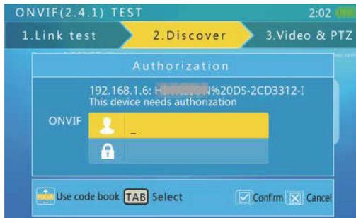
Use the flip keyboard to enter the user name and password, then press **Q** key to authenticate. On the interface of authentication, press **Q** keys to enter password interface. Figure:
