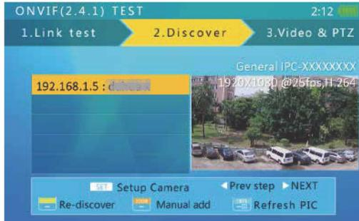
The top of the image will show the camera video resolution, refresh rate and the compression method.
