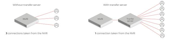
3) The Transfer Server will mirror all the devices assigned to it, so the "Quick Add" Device List will be fully populated as if the management server is in the same LAN as the IPCs.
