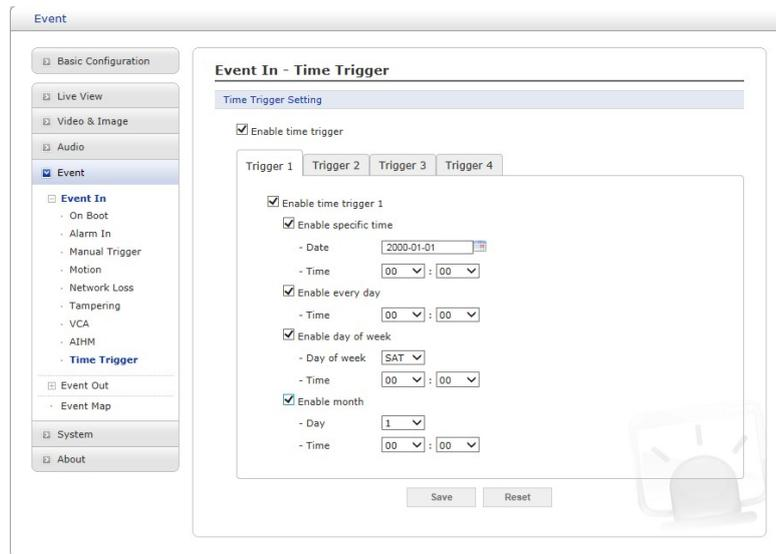
Time Trigger is to set alarms at specific time. User can set up to four time triggers and each time trigger can be set to specific date in the calendar, every day, day of the week, or date of every month.
