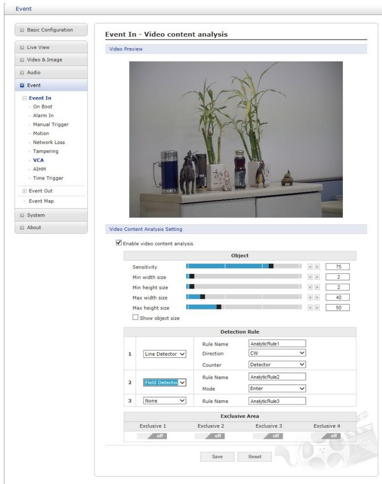
The network cameras provide VCA(Video Content Analysis) functions of “Line Detector” and “Field Detector.”
