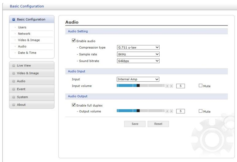
The network camera can transmit audio to other clients using an external microphone and can play audio received from other clients by attaching a speaker. User can setup and change setting of Audio in this page.
