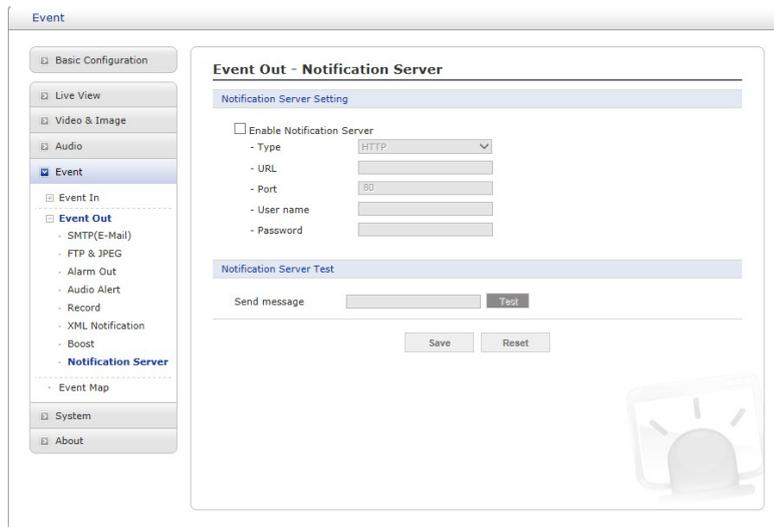
When the network camera detects an event, the Notification Server is used to receive up- loaded image files and/or notification messages. Check the box to enable the service.
