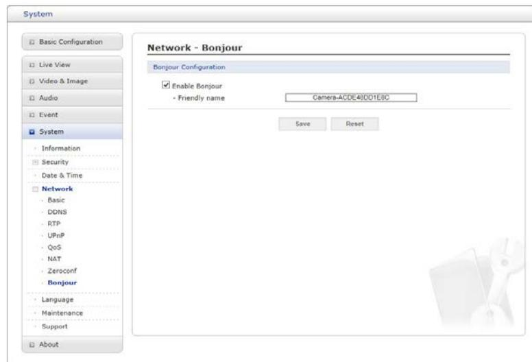
The network camera includes support for Bonjour. When enabled, the network camera is automatically detected by operating systems and clients that support this protocol.
