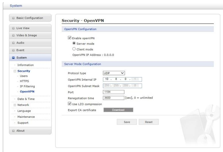
OpenVPN is a Virtual Private Network using OpenSSL authentication. User can set the camera in either Server mode or Client mode.
