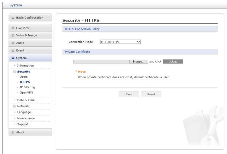
For greater security, the network camera can be configured to use HTTPS (Hypertext Transfer Protocol over SSL (Secure Socket Layer)). Then all communication that would otherwise go via HTTP will instead go via an encrypted HTTPS connection.
