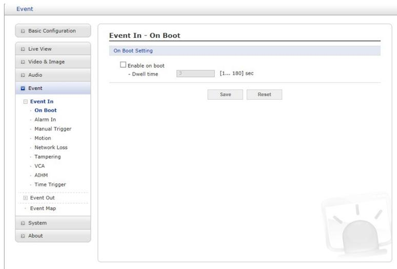
This is used to trigger an event every time the network camera is started. Select “Enable on boot” to activate the On Boot event.
