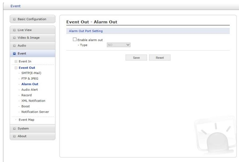
When the network camera detects an event, it can control external equipment connected to its alarm output port.
