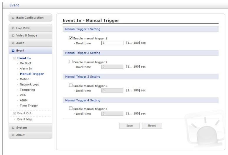
This option makes use of the manual trigger button provided on the Live View page, which is used to start or stop the event type manually. Alternatively, the event can be triggered via the product's API (Application Programming Interface).
