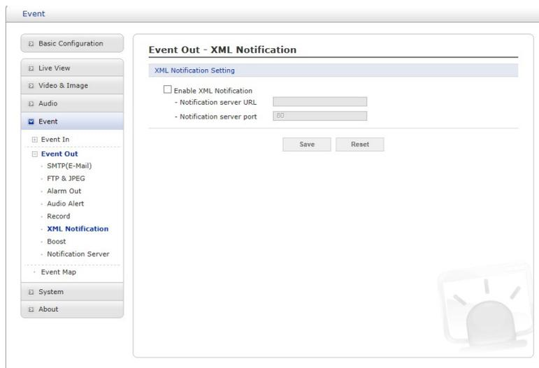
When the network camera detects an event, Notification server is used to receive notification messages as a type of XML data format. Check the box to enable the service.
