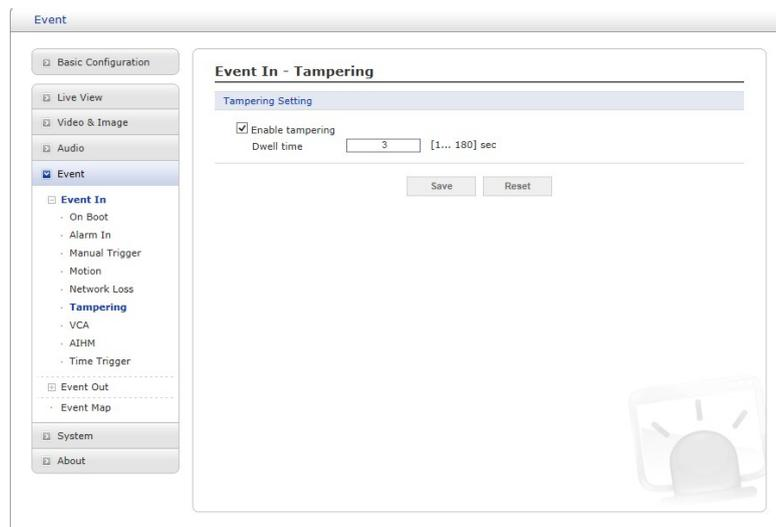
This is used to trigger an event when camera tampering occurs, for example, obstruct the camera with foreign material or move camera direction using external force.
