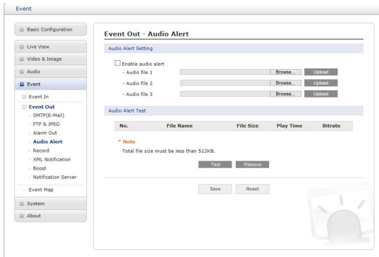
When the network camera detects an event, it can output a predefined audio data to external speaker. Check the “Enable audio alert” box to enable the service.
