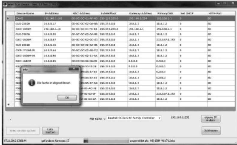
After pushing the button „Find eneo devices“ you will get a list of cameras connected to the local network. Highlight your camera in the list and open a context menu with a click of the right mouse button.
