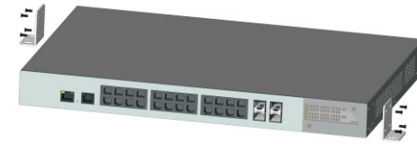
Figure 2-3 Hangers installation diagram
