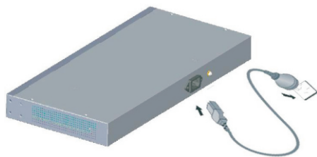
Figure 2-6 Connect power cable
