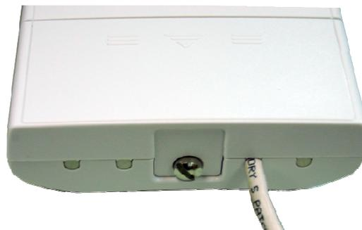
7. Power on the CDS-5IP - Wireless External Video Unit by plugging the power adapter to the power socket.
