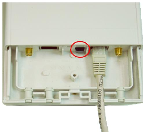
6. Attach and fasten the removable cover to the bottom of the unit with the screw.
