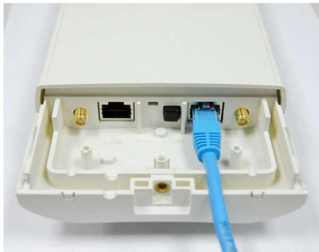
Figure 2 Cable Connection
