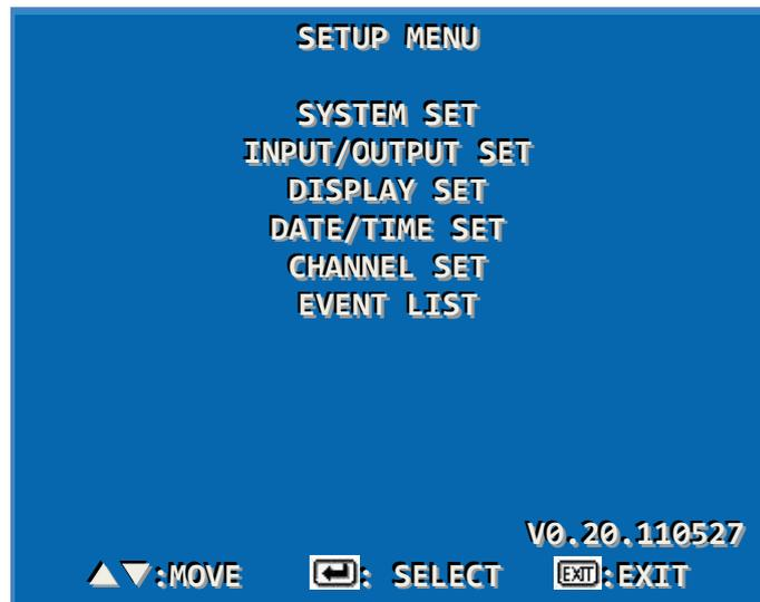
Button on front: Press the Menu > Press [ENTER] to select the mode by pressing ▲ ▼ buttons. > Press [ESC] to cancel or go back the previous menu.
