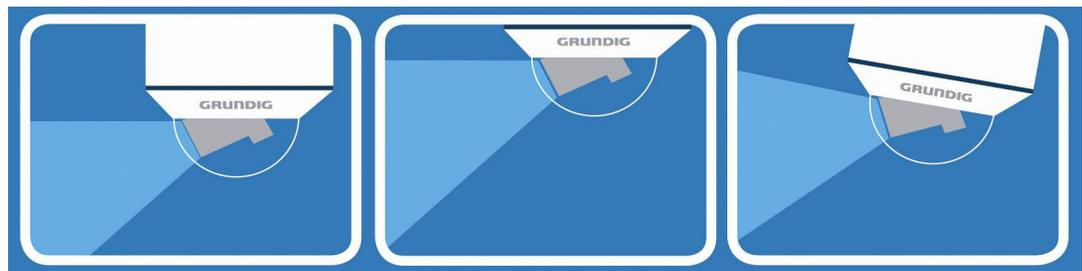
With standard bracket, Vandalproof dome allows only tangential view along the lid. The bracket enables inclined by increasing the angle of vision to monitor the wall supporting the camera. It is ideal for monitoring of ATMs, access, display cases.
