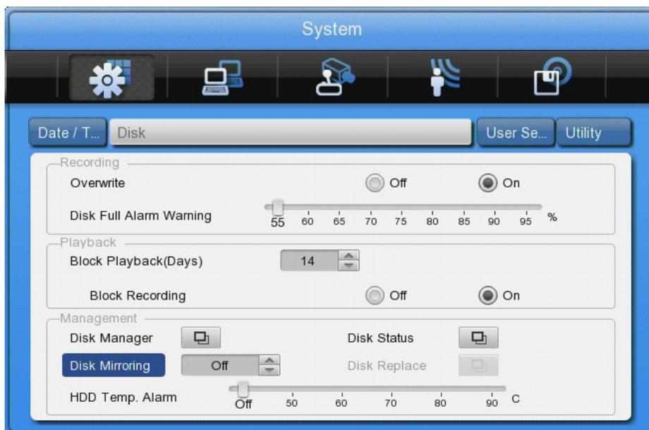
(4) To enable the mirror function, all HDDs need to be formatted. Select YES in the pop-up window to format the HDDs.
