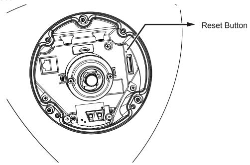
The reset button is used to reset the system or restore the factory default settings. Sometimes resetting the system can return the camera to normal operation. If the system problems remain after reset, restore the factory settings and install again.
