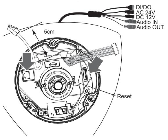
10. When cabling connection is done, secure the camera to bracket.
