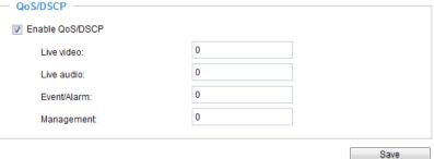
Note that different vendors of network devices might have different methodologies and unique implementations. Shown below is a sample corresponding information from a Cisco switch. You should enter a DSCP tag value according to the information provided by the network devices.
