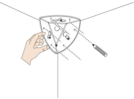
4. Drill 6 mounting holes (8mm in diameter) into the walls and ceiling. If preferred, drill a cable routing hole.
