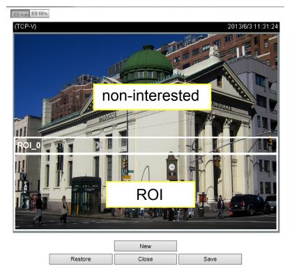
As the result, the lower screen is constantly displayed in high details, while the upper half (non-ROI) is transmitted using a lower-quality format. Although the upper half is transmitted using a lower quality format, you still have an awareness of what is happening on the whole screen.
