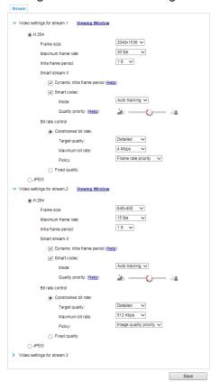
This Network Camera offers real-time H.264 and MJPEG compression standards (Triple Codec) for real-time viewing. If the H.264 mode is selected, the video is streamed via RTSP protocol. There are several parameters through which you can adjust the video performance:
