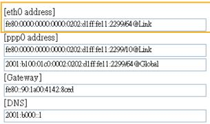
Manually setup the IP address: Select this option to manually set up IPv6 settings if your network environment does not have DHCPv6 server and router advertisements-enabled routers. If you check this item, the following blanks will be displayed for you to enter the corresponding information:
