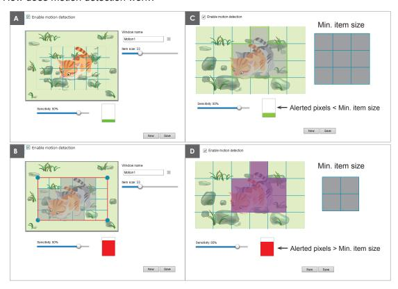
There are two motion detection parameters: Sensitivity and Min. Item Size. As illustrated above, frame A and frame B are two sequential images. Pixel differences between the two frames are detected and highlighted in gray in which the sensitivity setting will take effect. Sensitivity is a value that expresses the sensitivity to moving objects. A higher sensitivity setting allows camera to detect slight movements while a lower sensitivity setting will neglect them.
