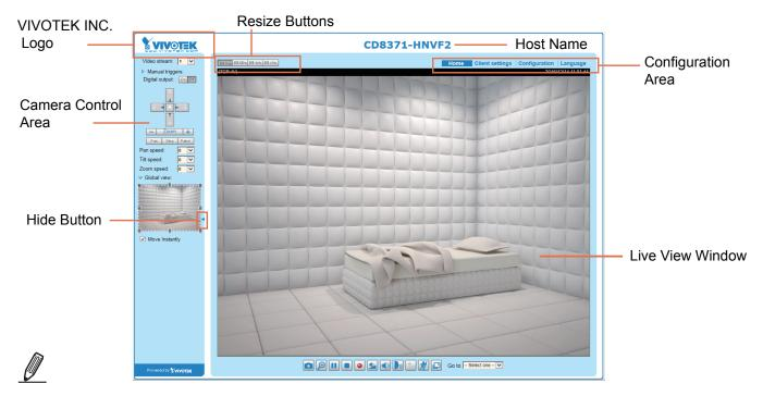
The Camera Control Area, the ePTZ control, is.only available for stream #3.
