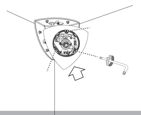
11. Insert a MicroSD card. Replace the desiccant bag with the one that comes with the shipping package.
