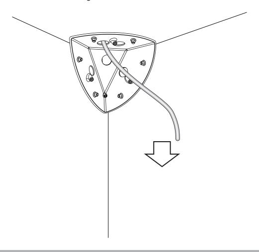
7. Install rubber gasket to the Ethernet cable. Pass the cable through the routing hole on camera and install the gasket.
