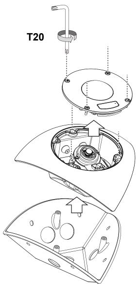
3. Use the base bracket as a template, and draw drill holes using a pencil. The camera is designed to be installed to a 3-sided corner of a room.
