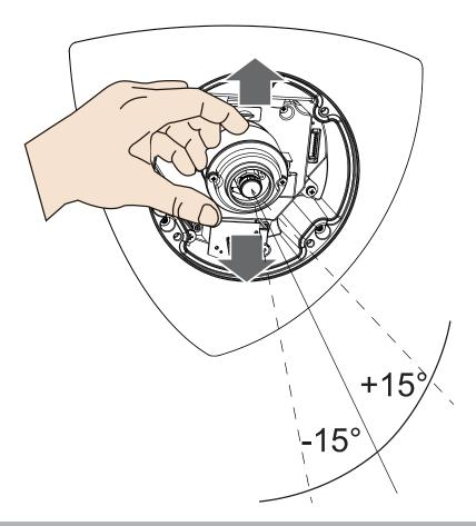
Adjust the lens module so that the field of view can cover the entire room.
